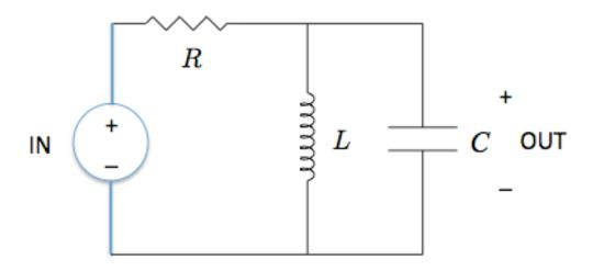
3) Consider the circuit below. The output is given by out2(t) . Find the state and then determine the state space representation.
