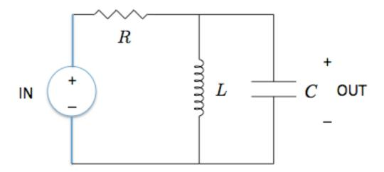
3) Consider the circuit below. The output is given by out(t). Find the state and then determine the state space representation.
